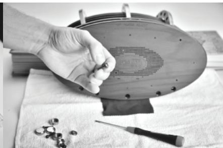
Place the clock to a soft towel showing its back to you and tilt it forward to access the bottom part
